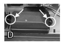
Reinstall wire cover and upper receiver box cover (add grease to foam pads on receiver box to ensure watertight seal).
